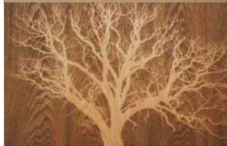
These digitally drawn trees are laser etched onto birch ply, or laser engraved onto oak-veneered MDF to create these stunning effects
